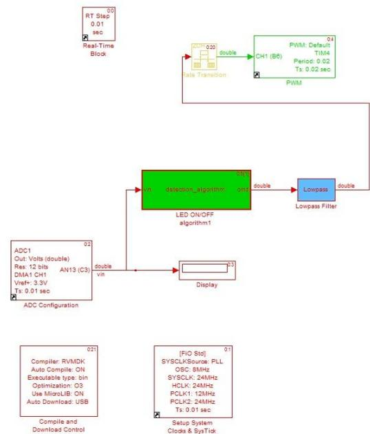
Fig.10: Simulink program of brake and accelerator systems
