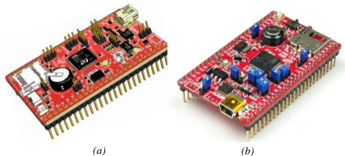
Fig.7: (a) CAD design of FiO Board (b) FiO Board Controller
