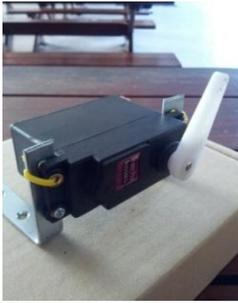
Fig.2: 9850MG Servo Motor from Towerpro
