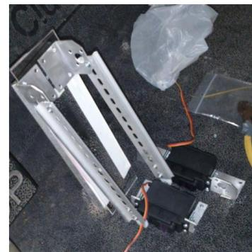
Fig.6: Mechanical part of accelerating system and brake
