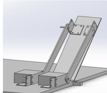
Fig.5: CAD design of Accelerator and brake systems
